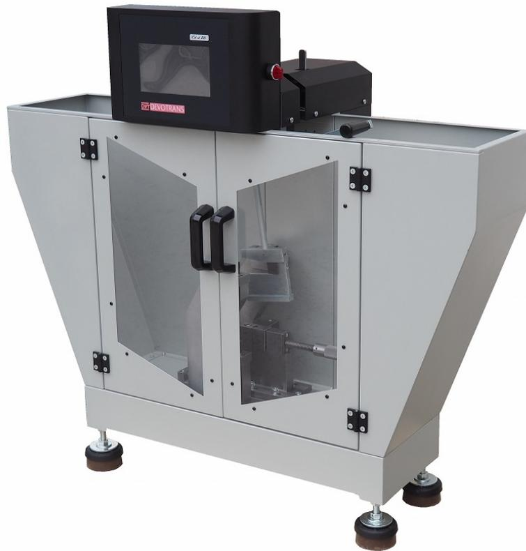
**USED TO DETERMINE BREAKING FORCE FOR PRODUCTS
